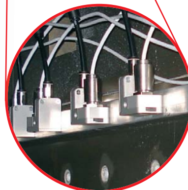
Picture 1: Small PSC CT LT sensing head; Heads installed in a machinery with laminar air purge collars for temperature monitoring during thermoforming
